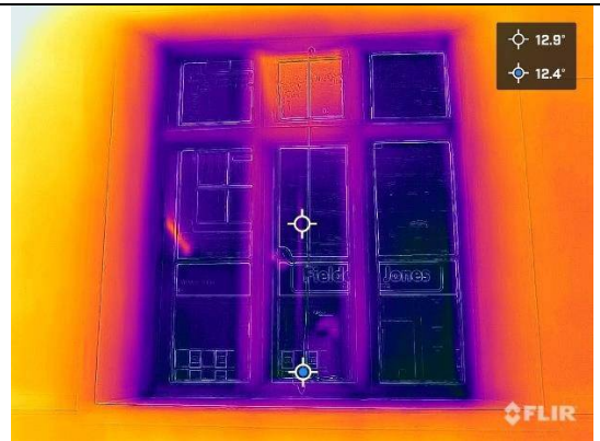
Figure 20: Example of retrofit double-glazed interior windows to reduce heat loss
